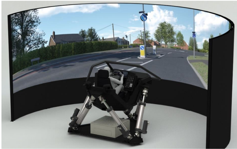
Figure 2.2: Layout of the motion base and the screen
